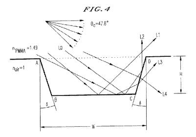
Figure 4 depicts scattering lights L1-L4 on the trapezoidal protruding pattern ABCD of an acrylic waveguide, including pattern width W, pattern height H, and slope angles  $\delta$ . (Col. 6, ll. 39-55).
